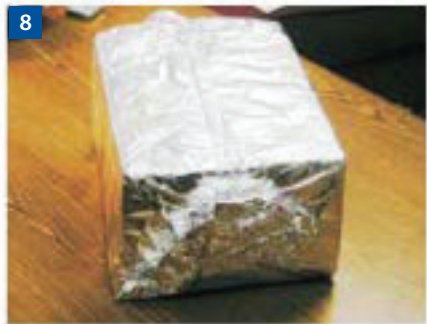
The finished foil wrapped sample should be tightly sealed on all sides. Remember: Only one sample per foil package.
