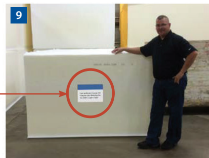
9 Take a photo of chemist or supervisor next to foam block from which sample was taken. Label the foam block with this information:
