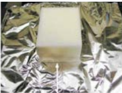
Place the foam sample in the center of the joined foil sheet lengthwise on top of the seam.
