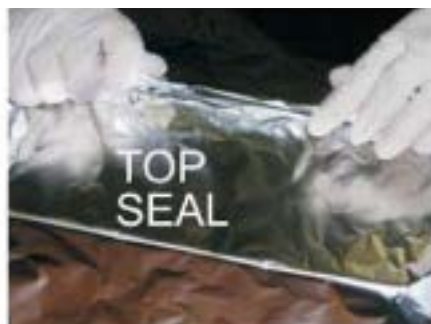
Join the side panels together at the top. Pinch the overlap, roll over twice and fold flat to seal.
