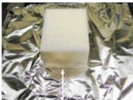
Place the foam sample in the center of the joined foil sheet lengthwise on top of the seam.
