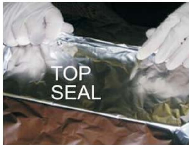
Join the side panels together at the top. Pinch the overlap, roll over twice and fold flat to seal.
